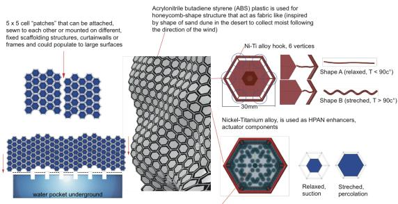
The material collects moist from air then condense into big droplets of water and passively transport them to the water pocket
