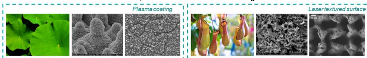
Fig.1: SEM images of hydrophobic plasma coating (left) and laser textured surface (right)
